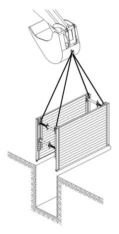
For trench depths greater than the base plate height, when applying the place and adjust method, base and top boxes must be assembled outside of the trench and placed into the trench as a whole.
