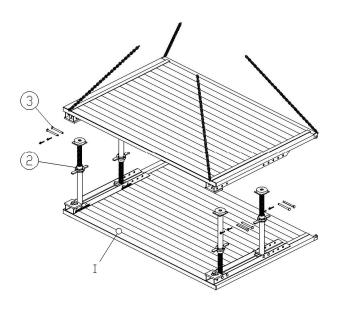
Put the base plates onto a flat and firm underground with the profile to the top.
