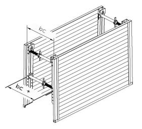
Now the struts are extended to the required trench width. (fine adjustment)
