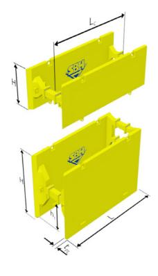
The Drag Box has been designed for trenches in the open air and with stable soils. Further excavation of soil takes place ahead, and the Drag Box is pulled through the excavated trench to the new working position.
