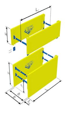
The robust, long-lasting Standard Box features a reinforced head, which can resist even the high loads when using the cut and lower method. At the same time, the reinforced cutting edge design enables even firm earth to be stripped away.
